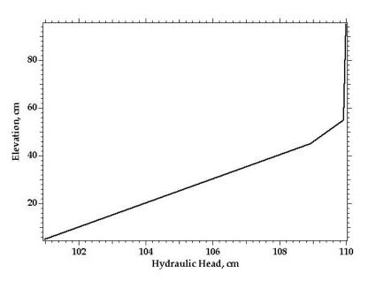
**Figure 6**. Flow in a saturated porous media column in response to a suddenly imposed 10-cm head (Silt hydraulic conductivity = 0.1 cm/day, Hydraulic head at 10 days).
