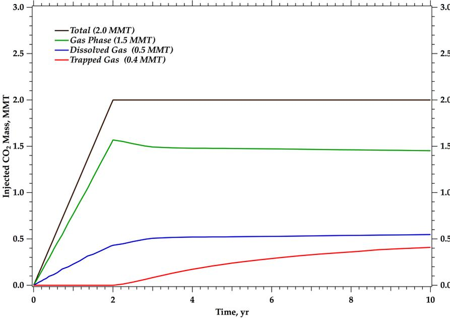
Figure 12. Integrated Mass of CO<sub>2</sub> vs. time
