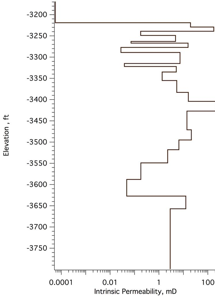
**Figure 2.** Vertical distribution of intrinsic permeability assigned to model layers
