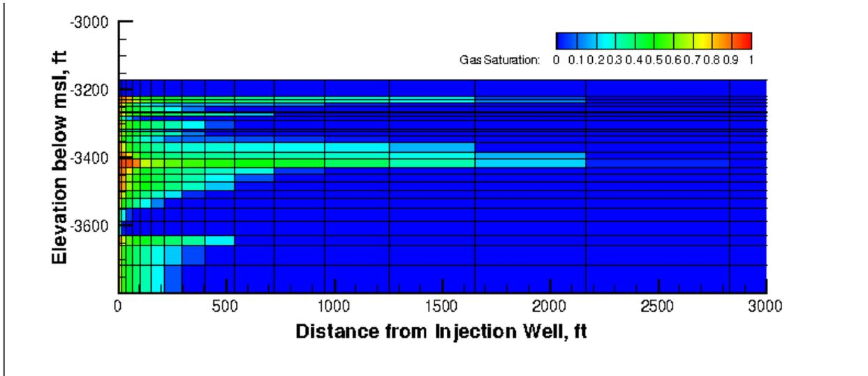
Figure 5. Gas saturation in the near field after 2 years of injection
