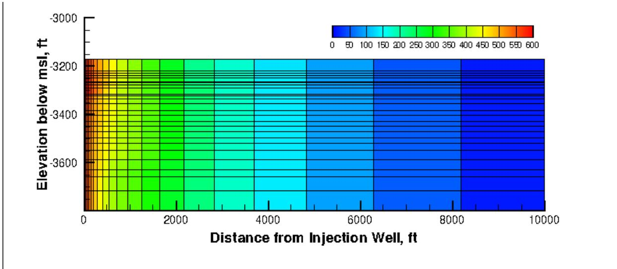
Figure 7. Pressure buildup (psi) in the reservoir after 2 years of injection
