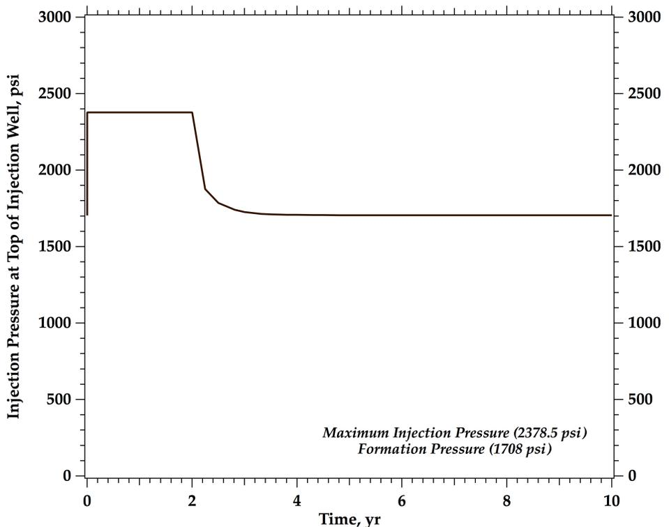
Figure 10. Injection Pressure at Top of Injection Well vs. time
