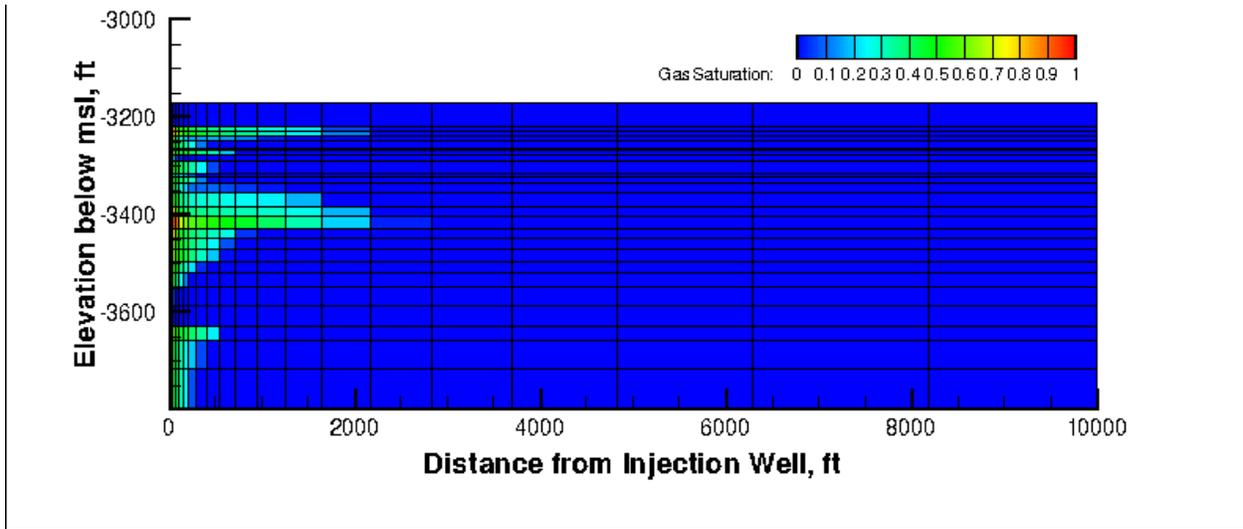
Figure 3. Gas saturation after 2 years of injection
