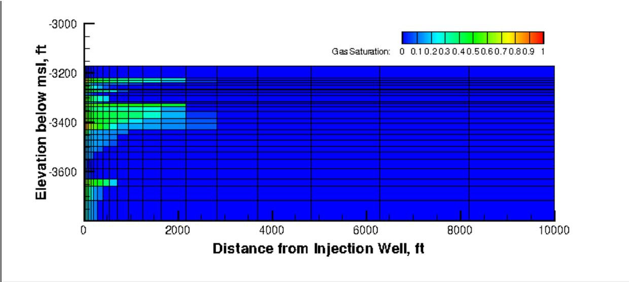
Figure 15. Gas saturation after 10 years of simulation time (2 years of injection and 8 years post-injection)
