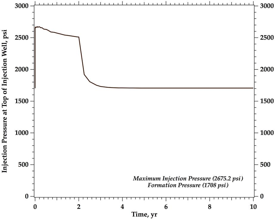
Figure 13. CO<sub>2</sub> Injection Pressure at Top of Injection Well vs. time
