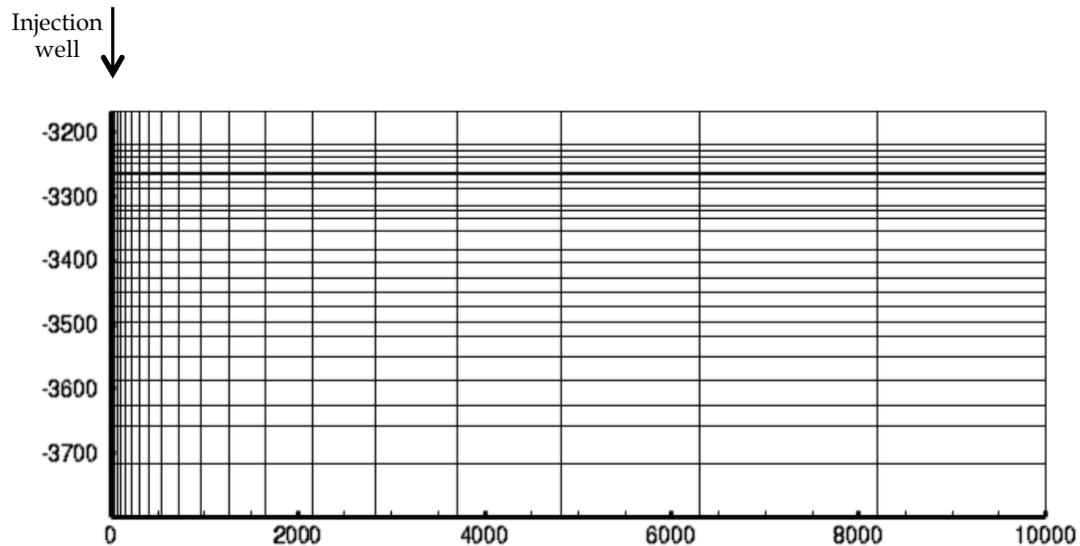
**Figure 1.** Grid for 2D (xz) slice of cylindrical domain
