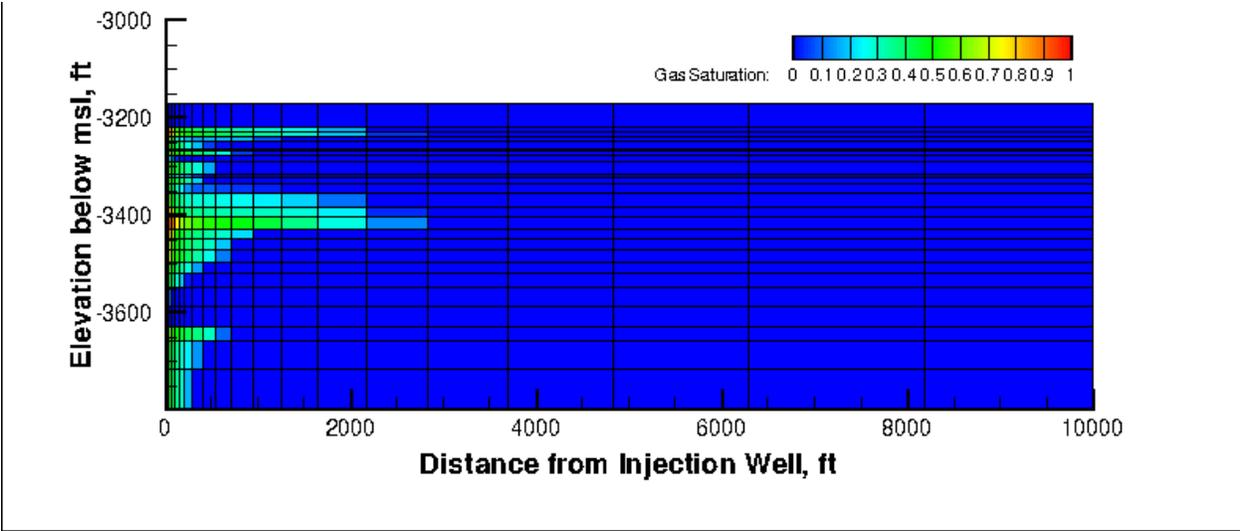
Figure 14. Gas saturation after 2 years of injection
