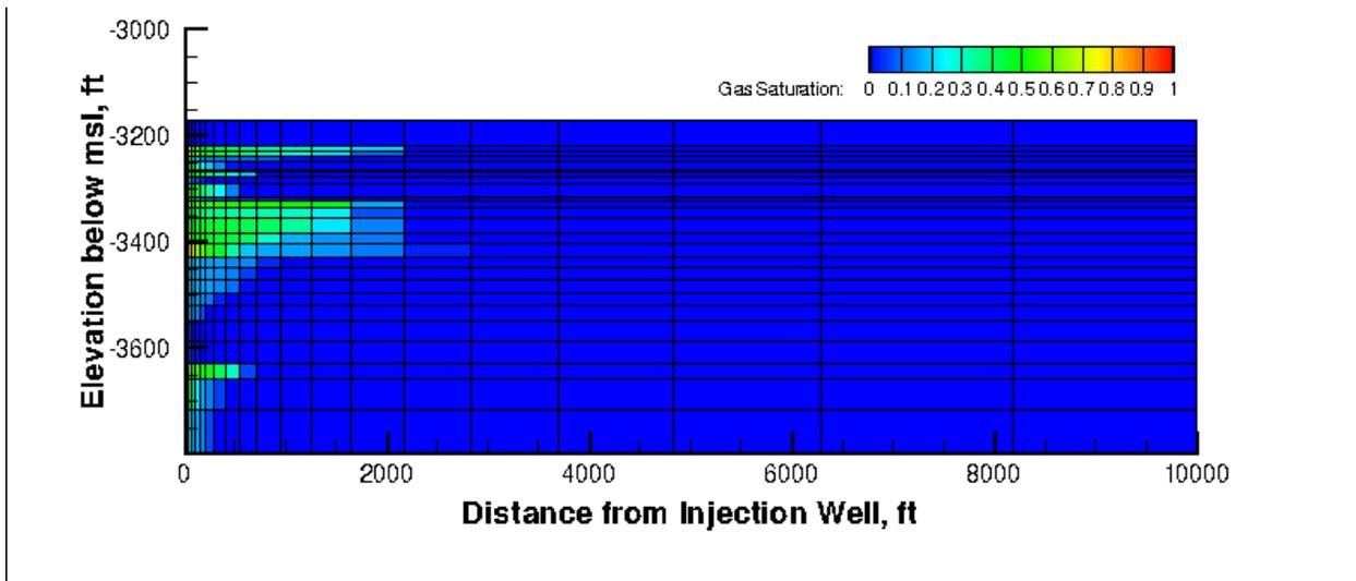
Figure 4. Gas saturation after 10 years of simulation time (2 year of injection and 8 years post-injection)
