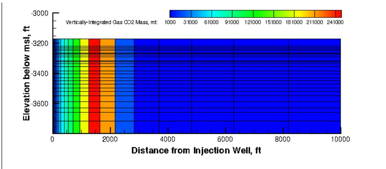
Figure 8. Vertically integrated mass of CO<sub>2</sub> in reservoir after 2 years of injection.
